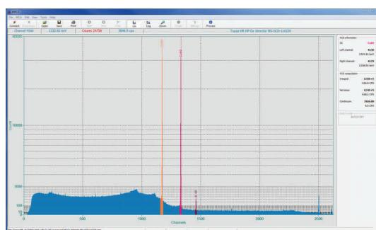
The Topaz-HR is an advanced, fully digital, compact Multi-Channel Analyzer. This device is used to process the electronic pulses typically produced by high-resolution semiconductor detectors such as Hyper-Pure germanium detectors (HPGe). However, the MCA can also be connected to other types of detectors, including scintillators (e.g. NaI(Tl), CeBr<sub>3</sub> or LaBr<sub>3</sub>, etc.), which makes it a valuable and multi-purpose device, a “must have” in your lab.
