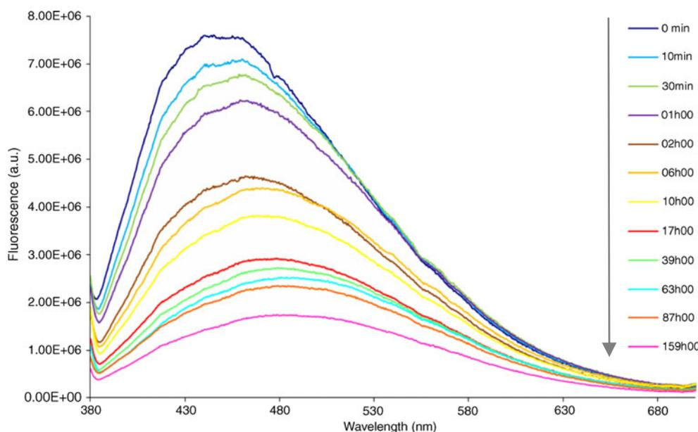
**Fig. 4** Normalized emission spectra of linseed oil before and after 313, 296 and 366 nm irradiations ( $T_0$ ,  $T_{17}$  and  $T_{159}$ )
