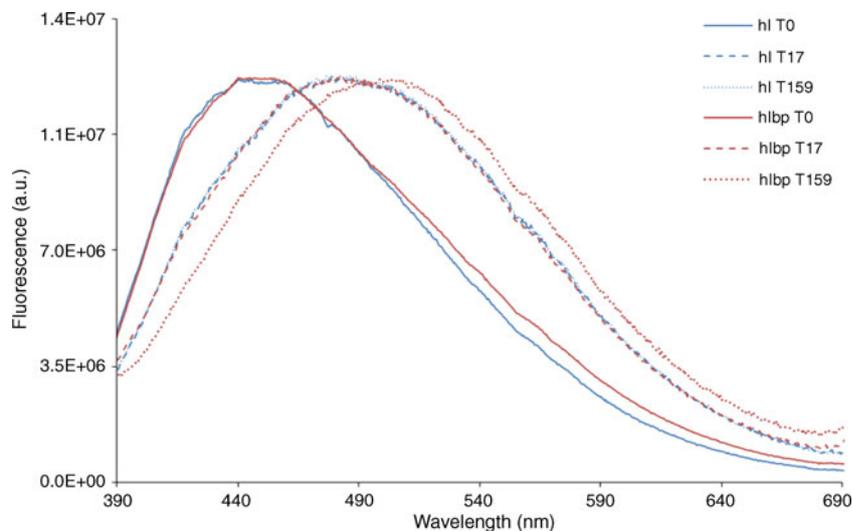
**Fig. 7** Emission spectra of linseed oil and linseed oil+lead white, on a glass slide and on limestone, before and after hydro-thermal ageing ( $V_{HT}$ ). Correction factors to normalized spectra are indicated (IF)
