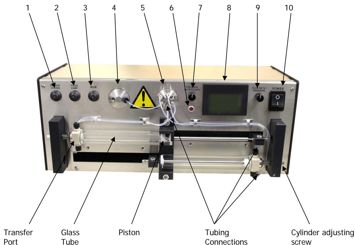
Figure 1 - DCP50 Front Panel with protective covers removed
