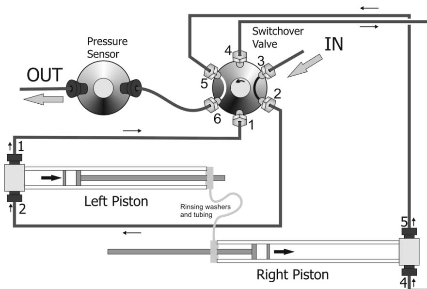
Figure 3 - Solvent Flow Diagram (including rinsing system)
