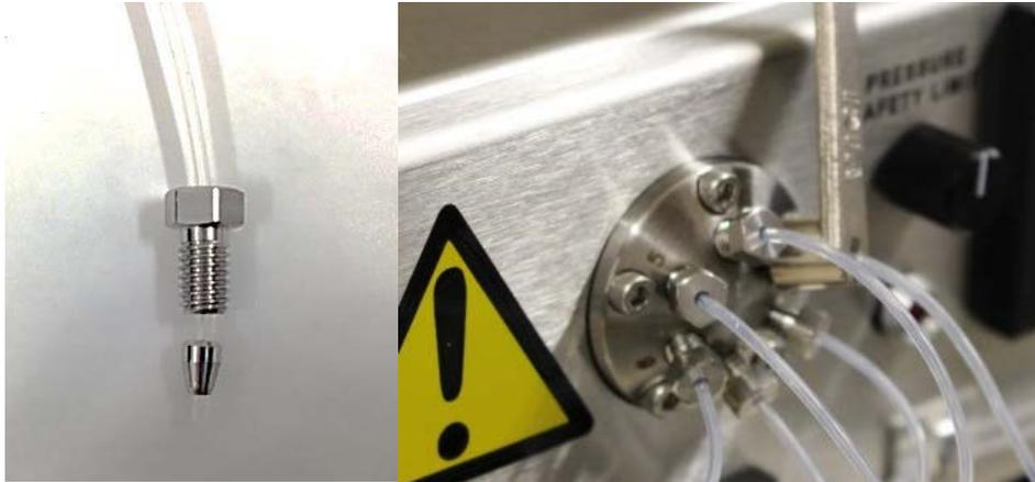
Figure 7 - Inlet tubing nut with ferrule (left) and wrench attached (right)
