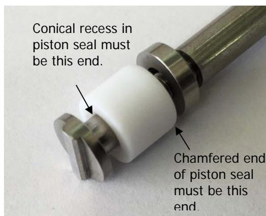
Figure 14 - Piston seal fitting
