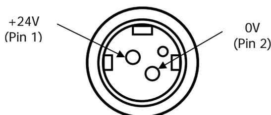
Figure 4 - DC Connector Pin-out (as viewed from rear of pump)
