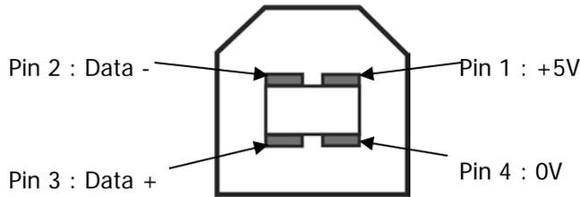
Figure 5 - USB Connector Pin-out (viewed from rear of pump)
