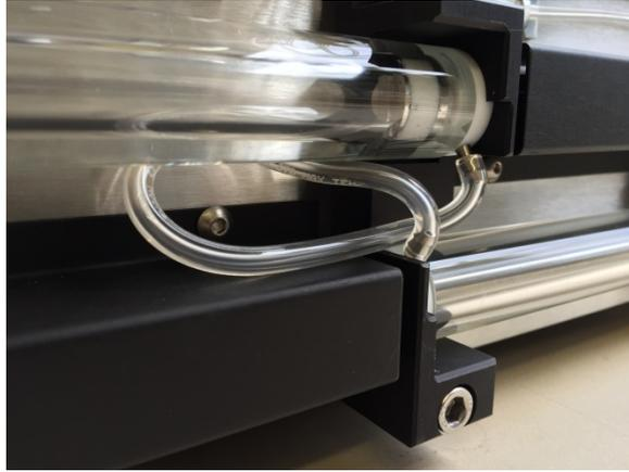
Figure 9 - Rinsing tubing in position
