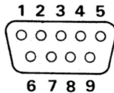
Figure 6 - RS485 Connector Pin-out (viewed from rear of pump)
