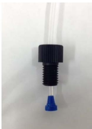
Figure 16 - Transfer port nut and ferrule
