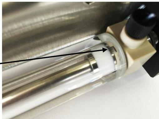
Figure 15 - Piston Seal Retainer alignment
